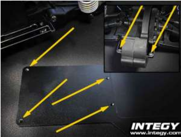
VI-1. Attach the modular rear end to the main chassis using four 3x6mm CS screws .
