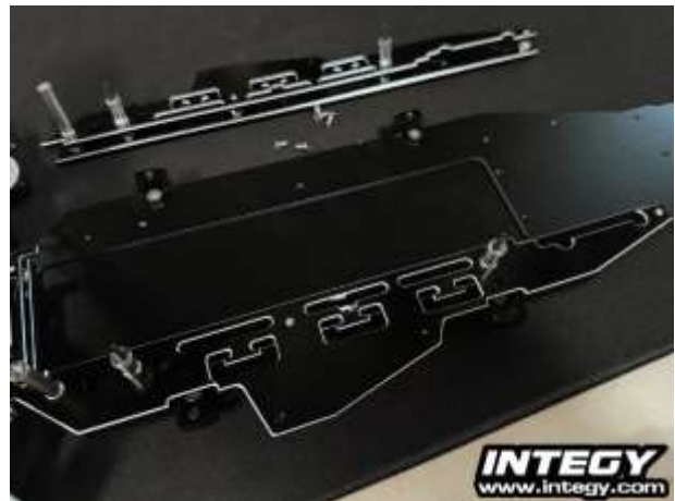
VI-4. Reinstall the modular side rails using 10 3x6mm CS screws (from Step V-1 to Step V-3 ).
