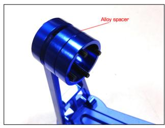
**4.** Attach the balancing assembly (the part with the ball bearings) to the balancer and tighten the four (4) 28mm button head cap screws.
