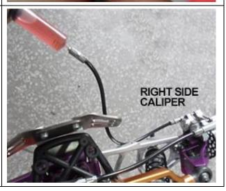
**6.** You will see some bubbles in the master cylinder reservoir along with brake fluid. Continue pressing the syringe plunger until no more air bubbles coming out with the fluid in the reservoir. Do not pull on the plunger at any time, or you will pull air into the lines and you'll have to restart the process.
