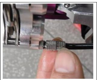
**4.** Using an open wrench, turn the hex-shaped filling nut ONE FULL TURN counter-clockwise.
