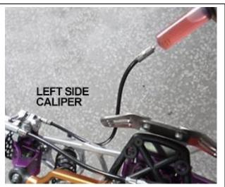
**10.** After filling the LEFT SIDE brake caliper with fluid, turn the hex-shaped filling nut ONE FULL TURN clockwise until the nut is tight.
