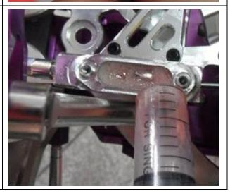
**12.** With one hand, move the master cylinder lever as shown to move the reservoir plunger outward. Add more brake fluid until the reservoir is filled flush to the top. After the reservoir is full, SLOWLY release the master cylinder lever.
