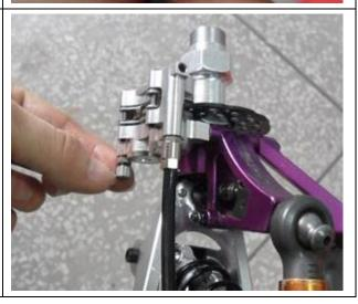
**9.** Using the second syringe, repeat steps 2-7 for the LEFT SIDE caliper. Don't forget to hold the syringe upright so that any air inside the syringe is at the top, and do not pull on the plunger at any time.
