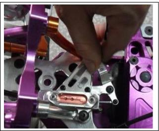
**13.** Reinstall the reservoir bladder into the reservoir. More brake fluid will spill out – this is okay, as you want to keep the reservoir as full as possible WITHOUT any air trapped inside.
