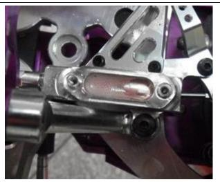
**7.** After filling the RIGHT SIDE brake caliper with fluid, turn the hex-shaped filling nut ONE FULL TURN clockwise until the nut is tight.
