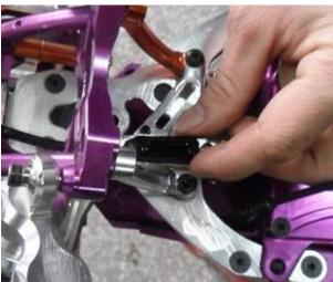
**14.** Finally, install the reservoir cap and mounting screws, and tighten the screws to secure the reservoir cap. At this point the hydraulic system is filled and bled, and ready to use.
