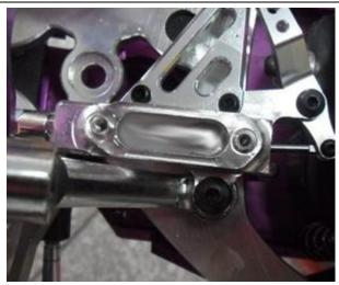
**2.** Prepare the RIGHT SIDE brake caliper for filling/bleeding by loosening the knurled filling cap located at the bottom of the caliper assembly counter-clockwise.
