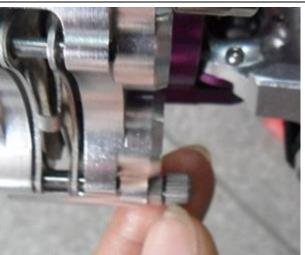
**3.** Get one of the filled syringes. Attach the filling hose to the brake caliper filling cap as shown, and tighten the nut snug (do not overtighten the hose fitting)
