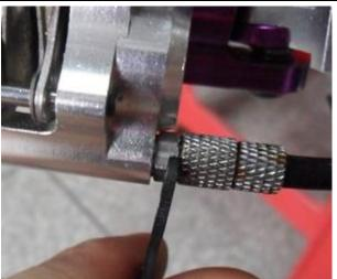
**5.** Hold the syringe upright so that any air inside the syringe is at the top. Slowly fill the RIGHT SIDE brake caliper with fluid. Stop when fluid begins to enter the master cylinder reservoir.
