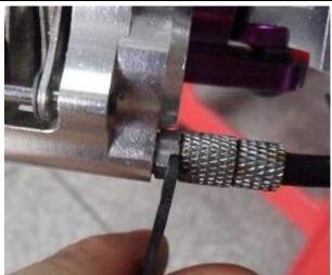
**8.** You can now disconnect the RIGHT SIDE syringe and hose. Don't forget to tighten the knurled filling cap clockwise.
