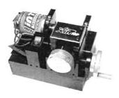
This machine comes standard with a carbide-cutting tool. It works well, but requires more frequent sharpening. The carbide-cutting tool will do a quality job, but it cannot match the finish of the cut or the durability you'll get from the optional diamond-cutting tool. Carbide replacement units are available from us directly. Also, we have developed a new type of diamond cutting tool (Xipp #90020) that cuts 3 times sharper than other diamond bits on the market.
