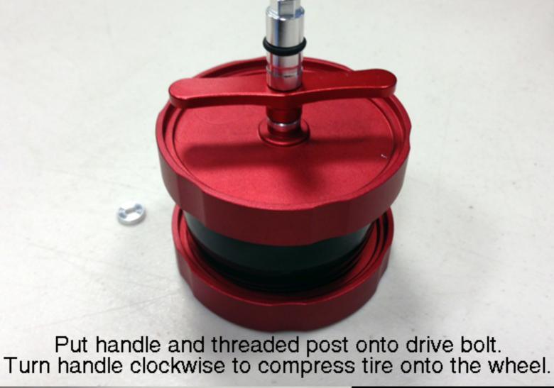
Turn handle clockwise to compress the onto the wheel.
