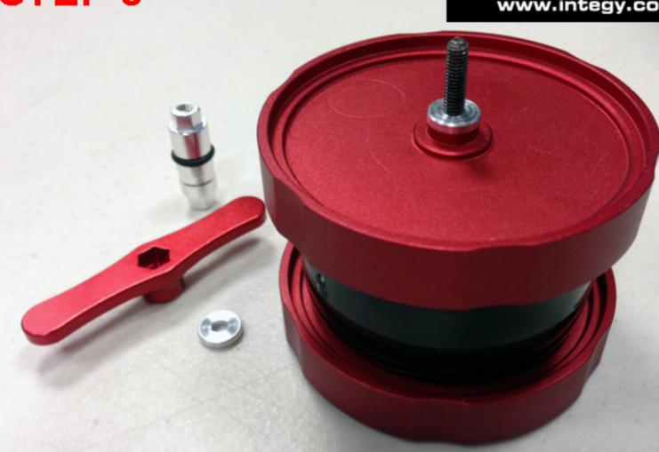
Place upper platform (flat side up, it's easier) and washer on drive bolt
