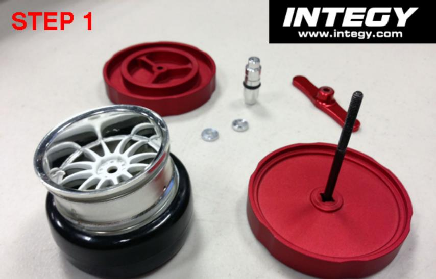
Insert drive bolt into lower platform (flat side up)
