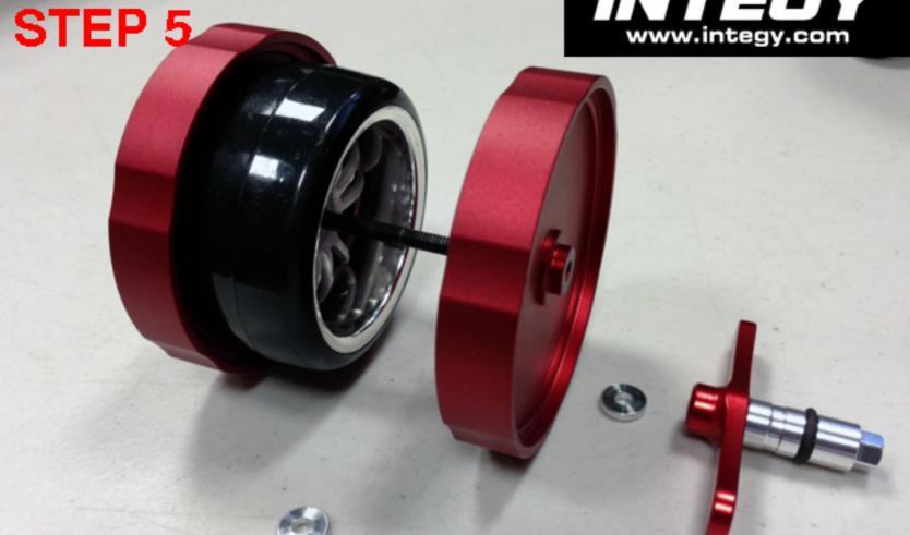
When you're done tire will be installed. Flip the platforms and do the same method to remove tire from wheel
