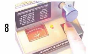
8 Hit the "Charge" button until the desired voltage is reached
