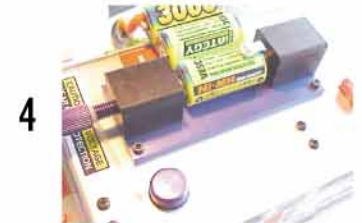
4 Install battery to cell holder (observe polarity)
