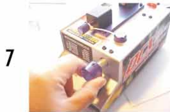
7 The "Arm" switch should now lock into position
