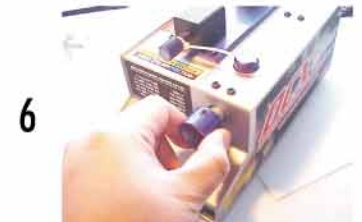
6 Twist and pull the "Arm" switch
