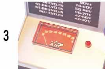
3 Make sure the meter reads zero volts
