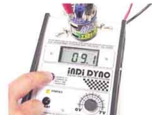
This motor draws 9.1 Amps during test
