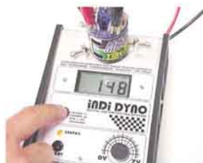
This motor is running at 14,800rpm
