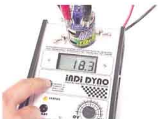
This motor has 18.3 interference index, which is pretty low for this type of motor
