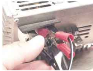
Connect Dyno to a 12VDC power source
