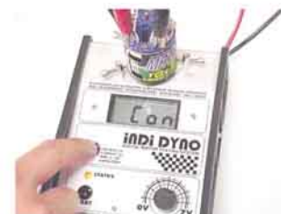
Con mode shows interference condition of your motor (lower usually is better)
